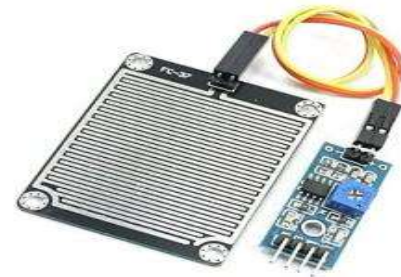
Figure-7: Raindrop sensor
